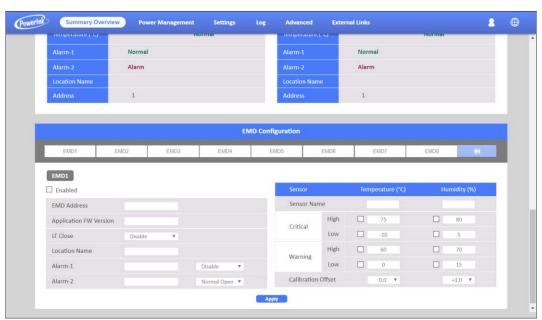
POWERTEK PDU supports 8 EMD sensors in cascade each one with 2 digital inputs to set 2 alarms for each EMD 31 sensor. There are 3 options(Normal Open/Normal Close/Disable) of the EMD sensor. If you set "Normal Open", the EMD sensor will become "Warning" (Yellow light) when closed.
