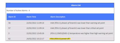
**Step 7:** The related log and trap will be recorded on the **Log** of **Event Log** webpage and NMS. The log and trap will be "warning: Inlet (PDU:1) Active/Main Power change to Active/Backup Power".
