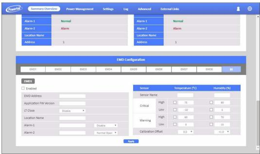
POWERTEK PDU supports 8 EMD sensors in cascade each one with 2 digital inputs of . you can set 2 alarms for each EMD sensor. There are 3 options(Normal Open/Normal Close/Disable) of the EMD sensor. If you set "Normal Open", the EMD sensor will become "Warning"(Yellow light) when closed.
